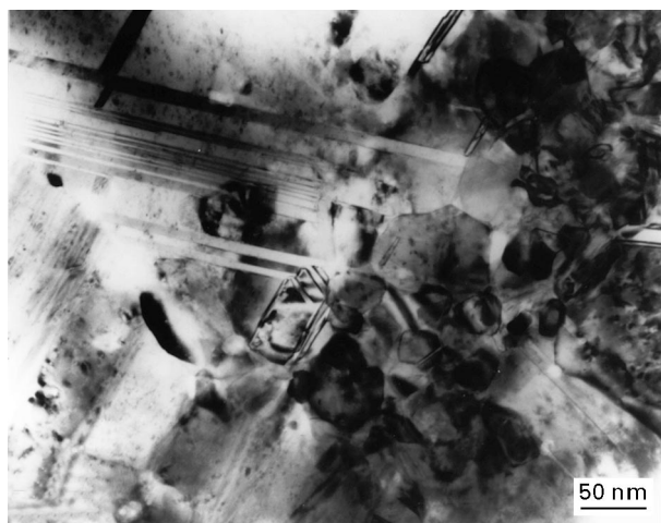
Figure 6 Bright field image of the specimens annealed at 200 °C. The compacting pressure of the specimen is 2.00 GPa.
