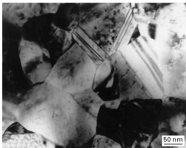
Figure 7 Bright field image of the specimens annealed at 400 °C. The compacting pressure of the specimen is 2.00 GPa.
